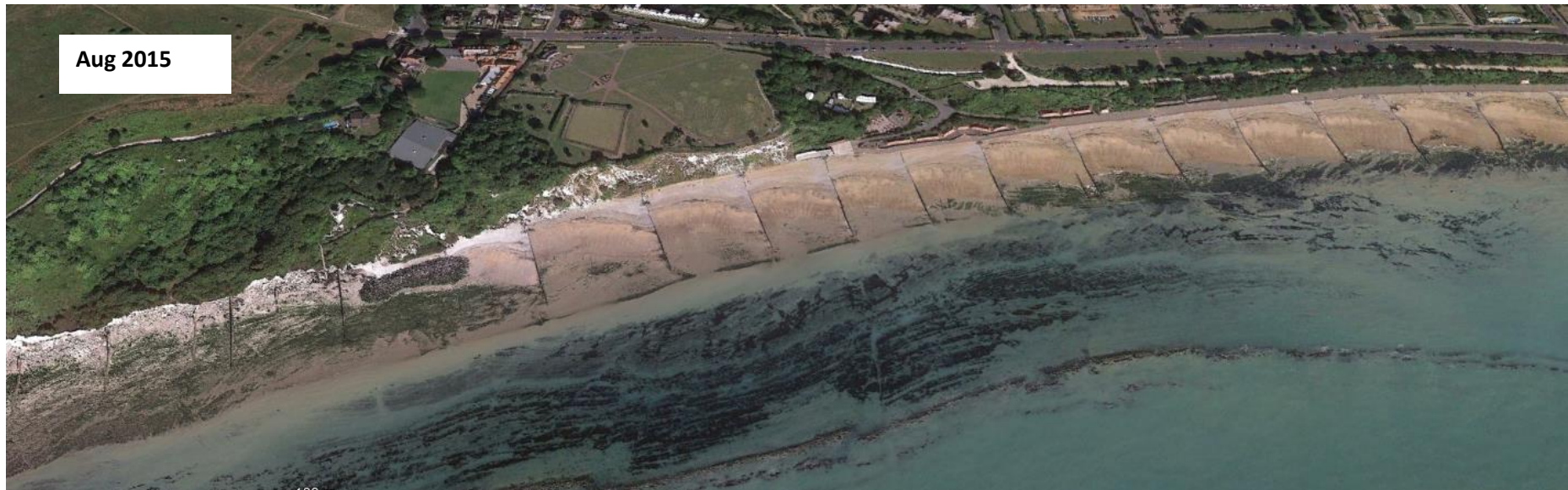
Figure 8: The beaches along the entire subject coastline between beachy Head and Cooden were subject to storms waves in May 2015, generated by 60 mph winds. The erosion pattern seen below the HW berms is evident along the entire 14km of subject coastline. There appears to be significant sediment loss due to draw-down and also longshore drift.
