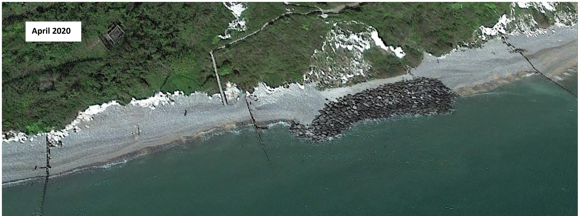
Figure 7: In just under 4 years a significant deposit of grey cobbles has drifted from the west to stabilise these beaches. These originated from the chalk scree deposits left on the beach following cliffs falls in 1999 and 2001.
