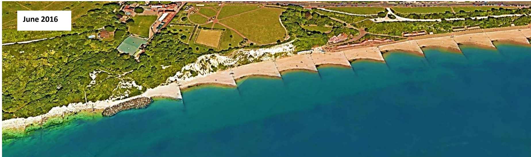
Figure 9: One year later the beaches appear to have been partially recharged with ballast. The beach plan-profile demonstrates the direction of longshore drift.
