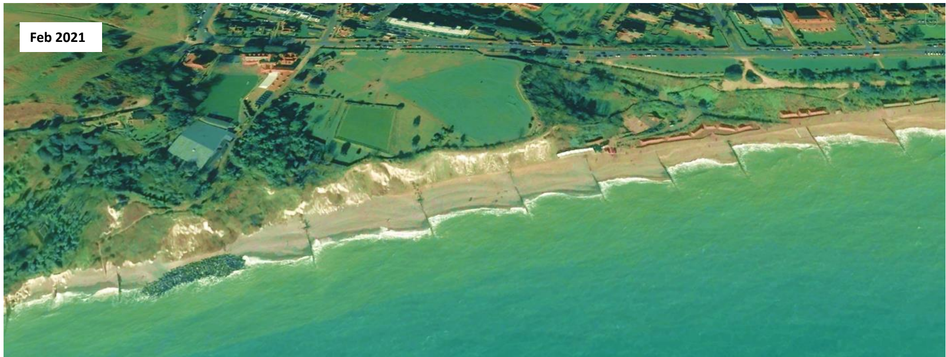
Figure 12: The grey cobbles and ballast have mixed within the high energy zone close to the HW berm and continue to drift eastwards and stabilise the beaches.
