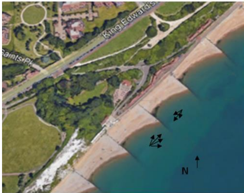
Figure 2: Beach profiles show the shingle stacking up against the northeast side of the beaches along Holywell. The vector arrows are extracted from wind roses. Image Google Earth.
